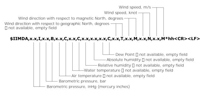
The fields related to quantities not measured by the instrument are empty (multiple consecutive commas appear to indicate the missing fields). The previous string is followed by a second string (**\$IIXDR...**) provided for measurements not implemented in these instruments.
