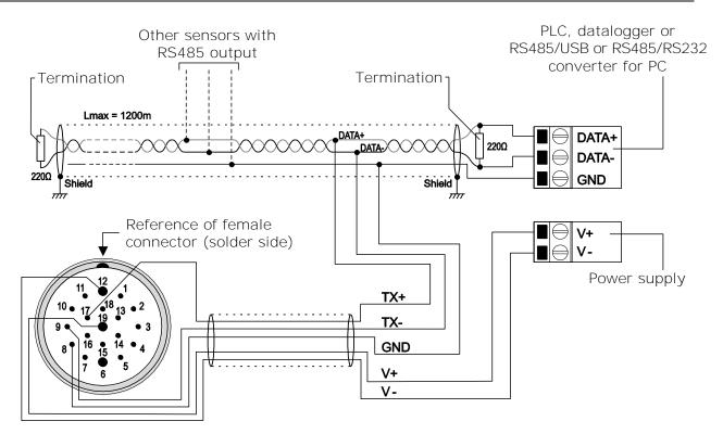
Thanks to RS485 connection, multiple instruments can be connected to a multi-point network. Instruments are connected in sequence through a twisted-pair shielded cable for signals and a third wire for ground.
