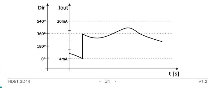
If 539.9° value is exceeded in extended mode, the output goes to the value corresponding to  $180^{\circ}$ .
