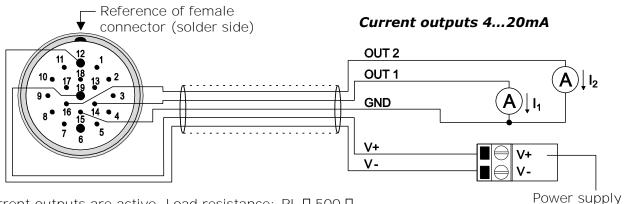
Current outputs are active. Load resistance: RL [] 500 [].
