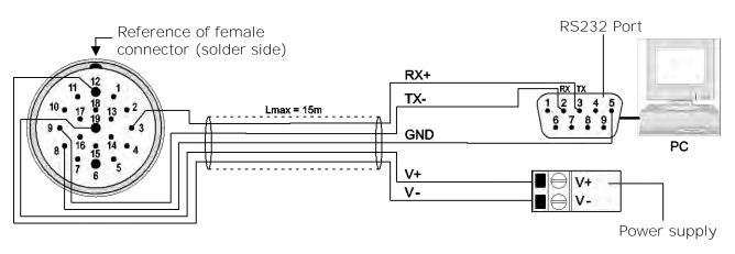
For RS232 connection, TX-, RX+ and serial GND signals (pin 9, 3 and 8 of M23 connector) are used, to be connected respectively to RX, TX and GND signals of RS232 port on PC (pin 2, 3 and 5 of 9-pole SubD connector). The length of RS232 cables should not exceed 15 m.
