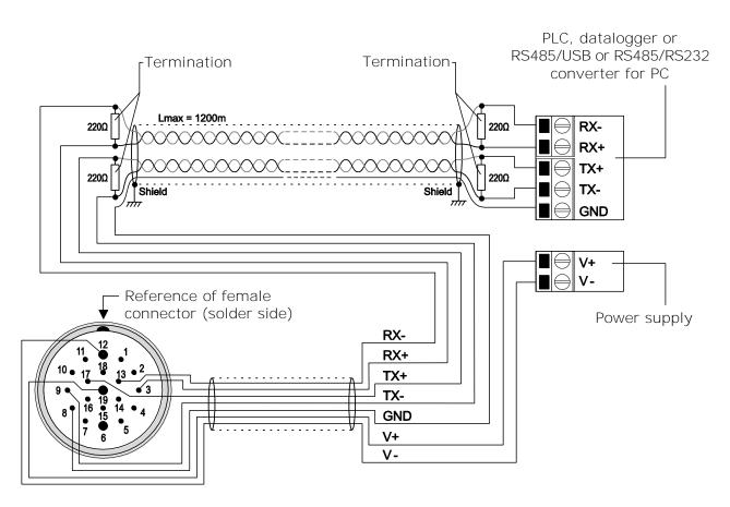
RS422 standard is used for point-to-point connection on long distances. The instrument is connected to a PC/data logger through a shielded cable with two twisted pairs for signals and an additional wire for ground. The extremities of the connections should end with line terminators.
