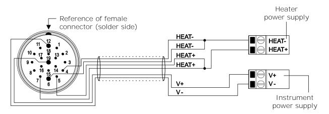
The heat circuit is switched on below +4 °C. After switching on, the heating is switched off when the temperature exceeds +10 °C.
