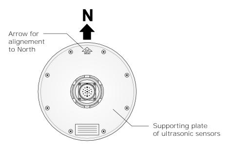
If a magnetic compass is used for alignment, take into account that the geographic North differs from the magnetic North indicated by the compass. The difference, named **magnetic declination**, depends on the area where the instrument was installed (for example, about 15° in North-America and less than 3° in Europe).
